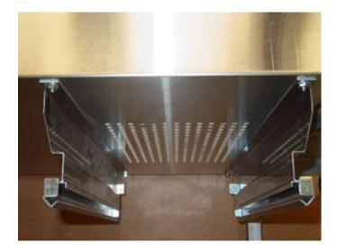
Position the CORN DRAWER SUPPORTS so that the CLEAN OUT DRAWERS may be slid between them, right beneath the table as shown. Screw the four CORN DRAWER SUPPORTS onto the table, each SUPPORT requires two 1/4-20 x 1/2 CARRIAGE BOLTS and two 1/4-20 SERRATED HEX FLANGE NUTS. Note: There are no washers needed. Insert the BOLTS from the top of the table, and tighten the HEX FLANGE NUTS on the SUPPORT sides.
